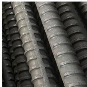
**Hot-rolled reinforcing steel with continuous thread ribbing\***, diameter 12-40 mm and up to 18m long, with exceptional features regarding toughness and ductility, particularly suitable for anti-seismic purposes and geotechnical works.
